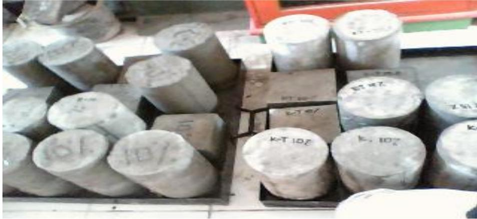
Gambar 4.12 Beton Uji
