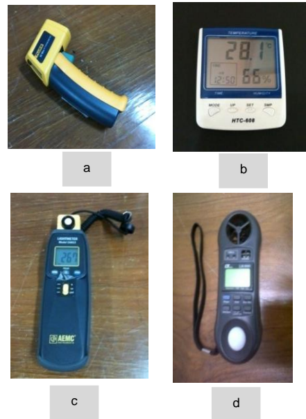
Gambar 12. Instrumen pengukuran, (a). Infra red thermo meter, (b). digital thermo-hygro meter, (c). lux meter, (d). 4 in 1 environment tester
