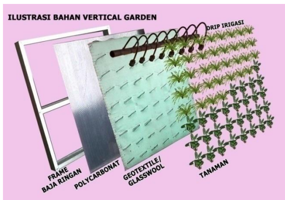
Gambar 3. Ilustrasi teknik vertical garden geotextile/glasswool
