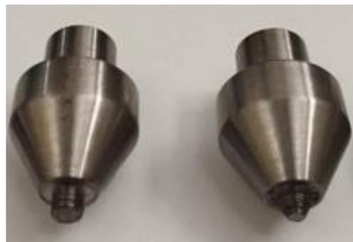
Gambar 10. Alat gesek FSW, (a) pin silinder berulir, (b) pin kerucut berulir
