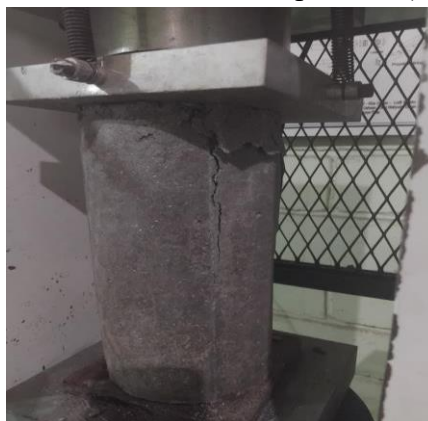
Figure 4. Broken concrete specimens after the compressive strength test
